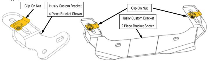
2. Install the 5/8"-11 hex head bolts & 5/8" hardware provided in the Husky Custom Bracket kit. DO NOT USE with a carriage bolt; you will NOT be able to tighten the bolt.
